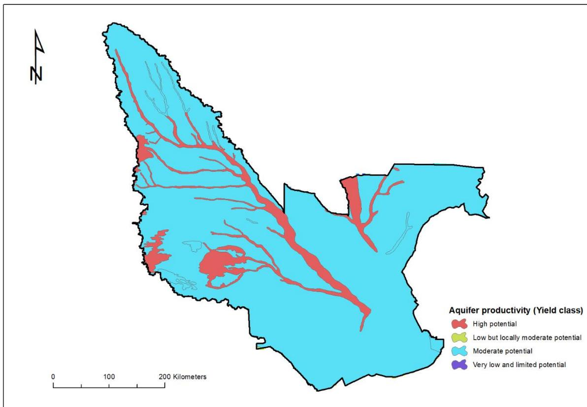
Figure 14: Aquifer productivity map from SADC hydrogeology map scale of 1:2,500 000 obtained from SADC-GMI (SADC, 2009)
