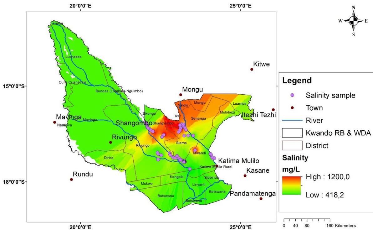
Figure 11: Salinity spatial values interpolated using Inverse Distance Weight based on combined wet and dry season sampling sites
